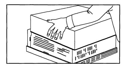
3. Select a suitable empty slot. You can install the card in any slot of an HP Vectra PC or an IBM PC or PC/AT. Choose a slot that gives good access to the HP-IB connector, but it's best to not place the interface next to a VGA card. You may install it in any slot of an IBM PC/XT except slot 1 (closest to the power supply).
