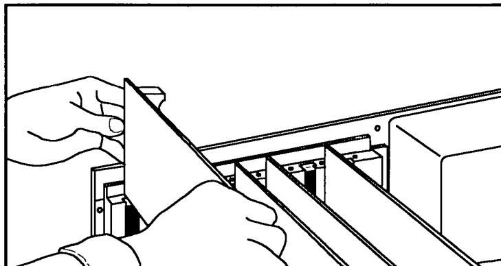
7. **Replace the slot cover screw** to hold the HP-IB interface in place. (Store the slot cover for use if the card is later removed from the computer.)
