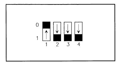
Choose an address (or select code) that isn't the same as the address (or select code) of any other card installed in your system. Select code 7 is the factory setting, which is most convenient for an HP Vectra computer—it's also required for the simple, default connection of a printer or plotter. Select codes 3, 5, and 6 are other common settings. If you have more than one HP-IB interface installed, each must be at a separate select code.
